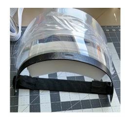
**Step 9:** Using an electric heavy duty stapler, staple each side as shown with three staples
