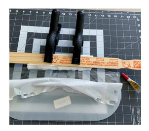
**Step 8:** Attach a 15.5 in. piece of high-strength (2 in.) elastic to the shield. Insert elastic from outside in through the side hole as shown – for no more than 2 in. Repeat on the other side as shown.
